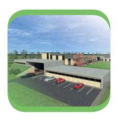
WWTP near residential area, 15 000 m³ treated water per day, 100 000 PE, recycled treated water in a thermal power plant, MBR
